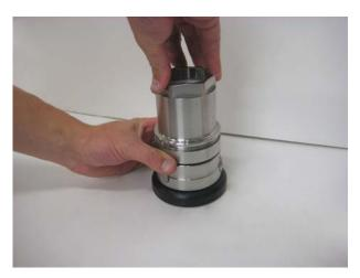
Place the swivel sleeve over the coupling body and screw in the swivel sleeve. The swivel ring has to be fixated as earlier when unscrewing the swivel sleeve from the swivel ring.
