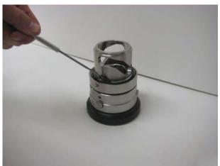
Remove and change the O-ring (pos.24) from the groove in the coupling body. Use grease on the new part. Apply grease on the balls for best possible swivel rotation.
