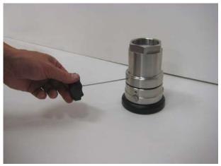
Unscrew and remove the lock screw from the swivel ring.
