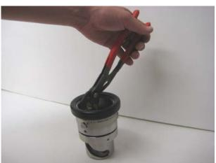
Press down the piston and turn the driving plate to the position where the recess ends up under the rollers.
