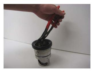
Press down and turn the driving plate to the position where the driving plate heels are placed under the rollers.
