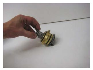
Press down the O-ring with your thumb. Make sure that the O-ring fits into the groove.
