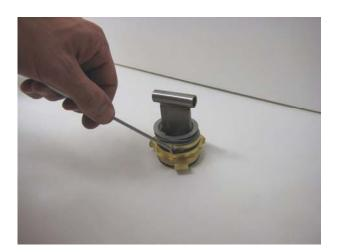
Change the O-ring (pos.8) on the driving plate back side. Use grease on the O-ring.
