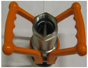
Finally, make a visual inspection that everything is in it's place. Do also a test connection / disconnection with a tank unit that not has any fluid inside. If the coupling works alright you are ready to mount the hose unit on your hose again.
