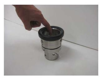
Change the three shafts (pos.18) and rollers (pos.17) to new ones.
