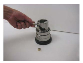
Mount the rolling shaft and the two rollers into the piston guide.
