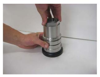
To unscrew and remove swivel sleeve from swivel ring. The swivel ring has to be fixated with help of an Ø6 mm pin.
