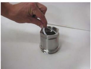
Place a new flat seal (pos.29) on the swivel sleeve. (Not needed when NPT-thread)
