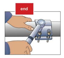
Straub couplings eliminate the need for threading, flanging, galling, and welding. Coupling installation takes minutes instead of hours.
