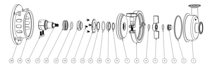
Any components that show signs of severe wear or damage should be replaced during the scheduled maintenance time for the equipment. Please refer to the assembly and disassembly section of this manual for proper instructions on removing and replacing any worn or damaged components. Replacement components and repair kits can be found in the BOM or repair kits section of this manual.
