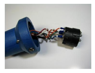
Per the picture above, slide the contact block out of the rack plug body. Slide the orange cord into the plug body as the contact block is slid out.
