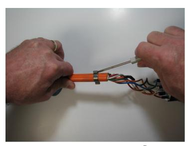
You can now remove the contact block from the cord. To remove the cord from the plug body you can loosen the clamp (see picture above) by inserting a screw driver in the crimped ears and twisting, or you can cut the cord off below the clamp so the cord can be removed through the strain relief.
