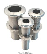
Specifically designed for underwater applications, the Arctic Steel Thru Hull fittings are cast in duplex 2205 stainless steel. These are unique in the marine market, providing much higher resistance to corrosion than regular 316, they are also significantly stronger than 316 and bronze making them ideal for a critical hull penetration fitting.
