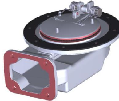
Emergency Foot Valves are installed in the floor of each tanker compartment and allow the inflow and discharge of fluid during the loading and unloading process of road tankers.
