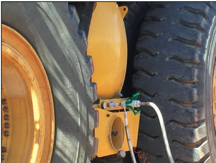
LNG fueling application on off-highway mining truck
